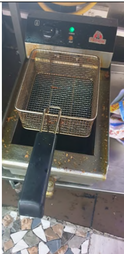
Staining and grease accumulation in deep fryer
