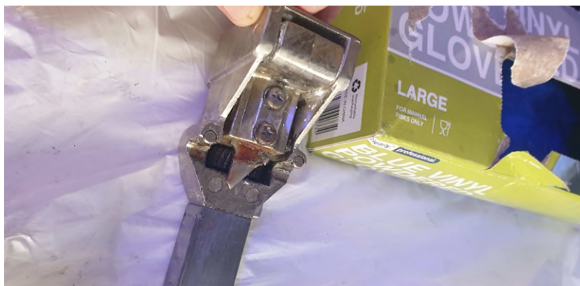
Food debris on the blade of can opener
